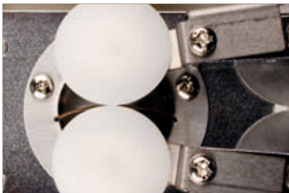
Large, especially supported guide rollers enable grooving of even difficult shapes
